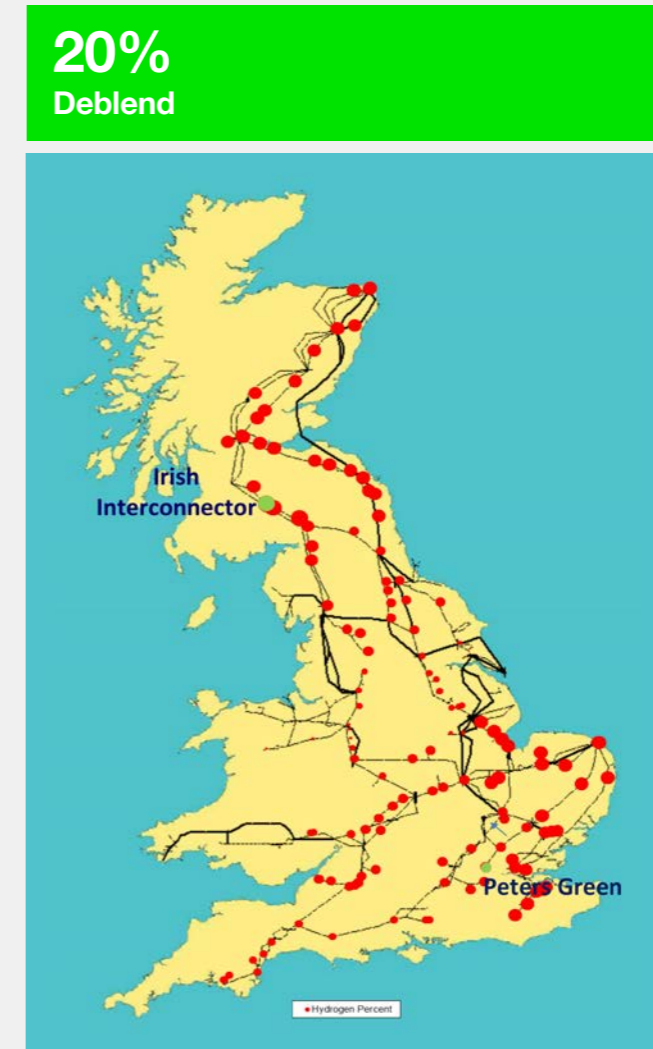
Figure 8 20% hydrogen blend in the NTS. Deblend at Irish Connector and Peters Green
